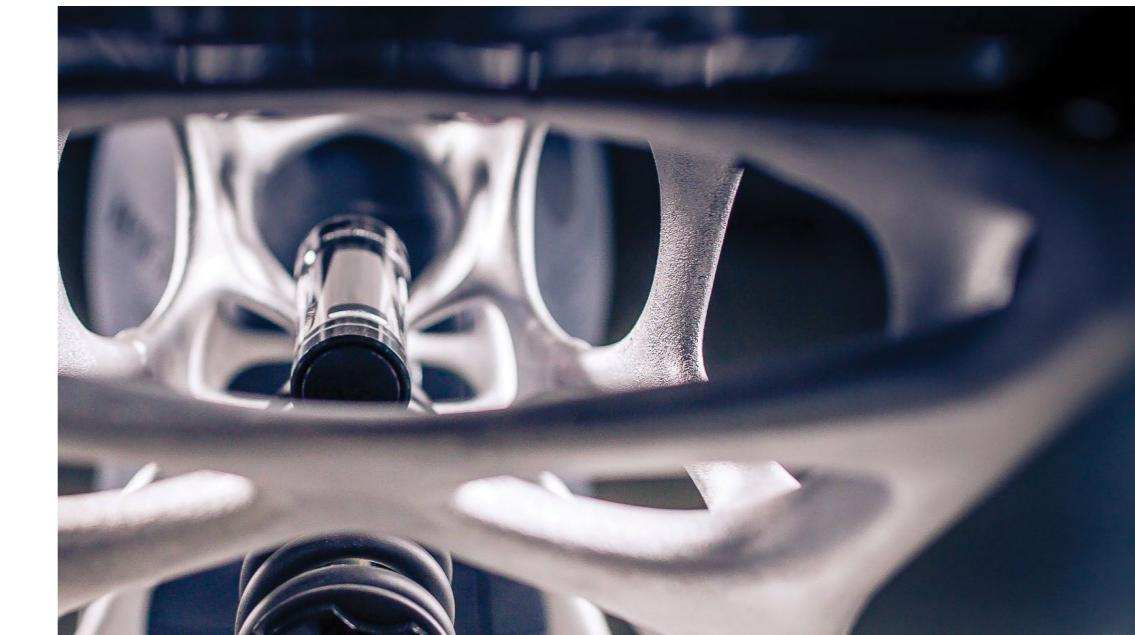
**Improving the reality** / By **topological optimizing** we can find the project solution that provides the best performance based on the project goals, starting from a predefined volume and the boundary conditions (constraints and loads).
